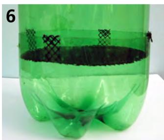
side through the overlapping layers of plastic with a small hot nail. Push a 140 mm length of garden wire right through to hold the two sections firmly in place. Make two more opposite holes with a larger nail (a 4-inch nail will give holes about 5 mm diameter) (Fig 7). Gently separate the bottle sections and twist by about 1.5 cm then push the small heated nail back through the hole in the outer bottle section so that there is now a second retaining hole in the inner section (Fig 8).
